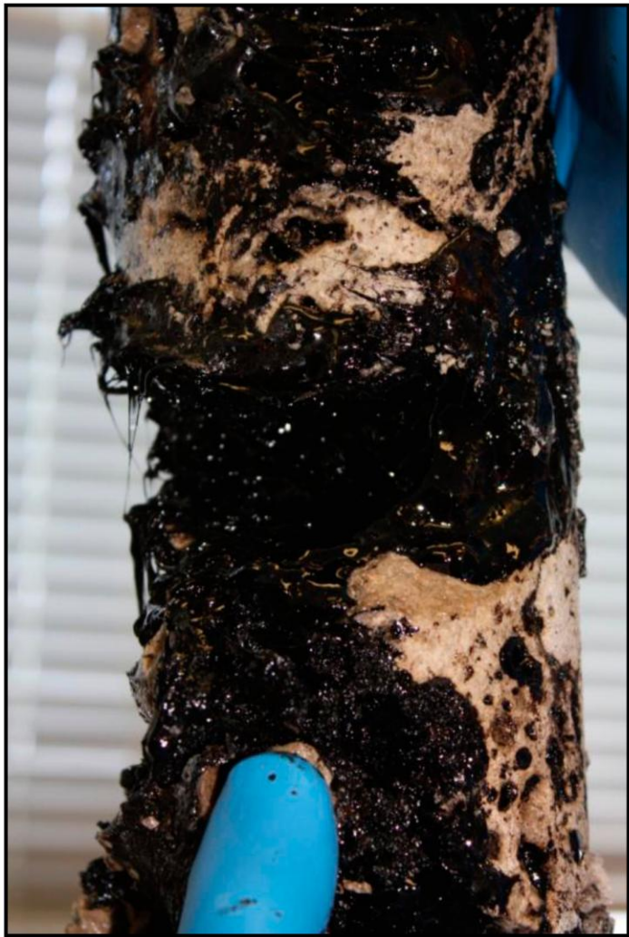
Figure 2. Core photos of the Leduc Formation showing (a) vuggy porosity, (b) bitumen filled fracture, and (c) bitumen recovered from a “cave”.
