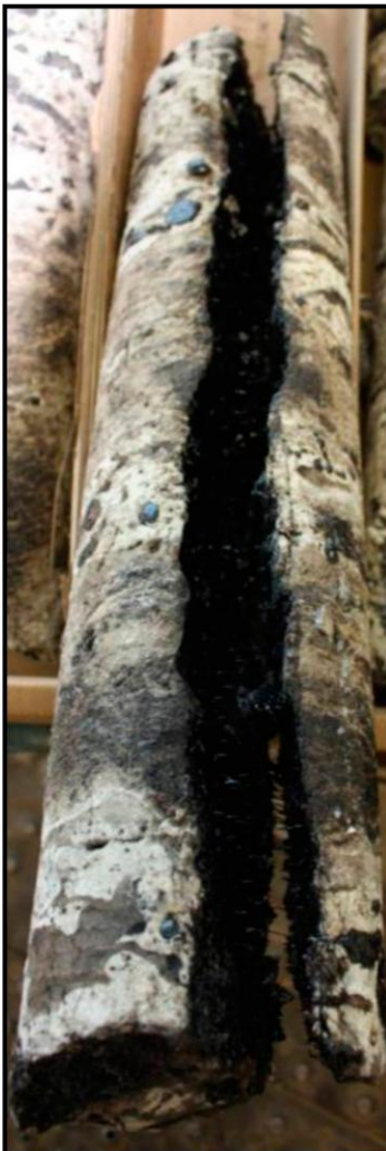
Figure 2. Core photos of the Leduc Formation showing (a) vuggy porosity, (b) bitumen filled fracture, and (c) bitumen recovered from a “cave”.
