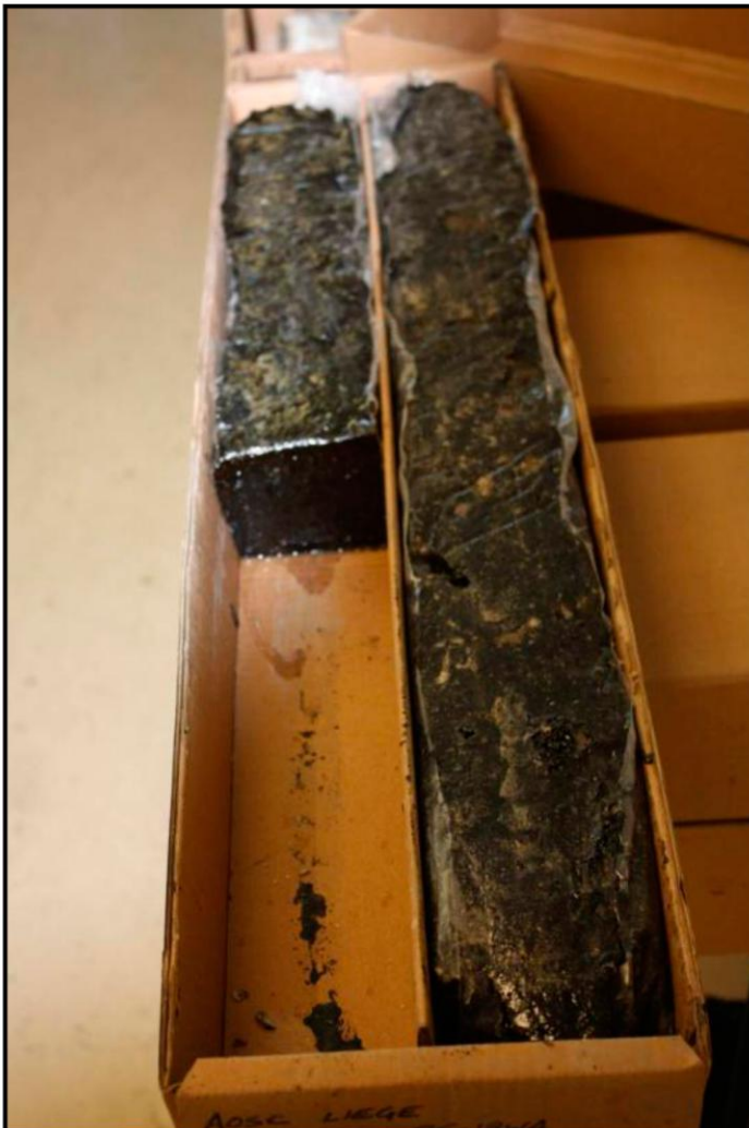
Figure 2. Core photos of the Leduc Formation showing (a) vuggy porosity, (b) bitumen filled fracture, and (c) bitumen recovered from a “cave”.
