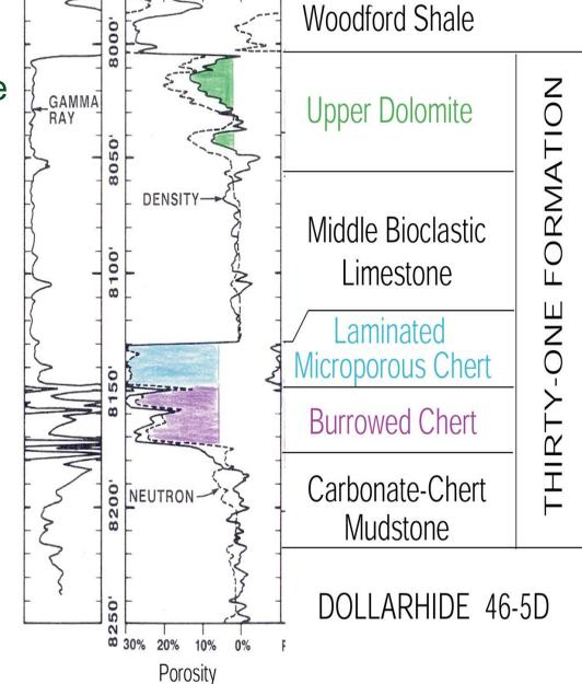
•Burrowed Chert - Burrowed Mixture of Sponge Spicules, Siliceous Mud, & Carbonate Mud Deposited in Broad Areas between Fans and Channels
