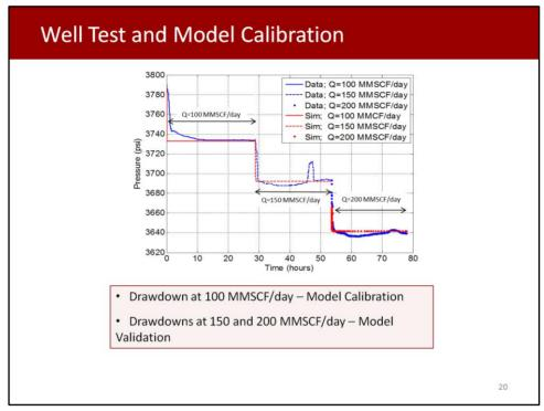
Presenter's notes: This plot shows the pressure drawdown observed during a flow after flow well test performed over a period of 80 hours, at 3 different flow rates of 100, 150 and 200 MMSCF/day. The blue line represents the actual drawdown observed while the red line represents the simulated pressure drawdown. The match is good enough for us to consider the fracture flow properties calibrated.
