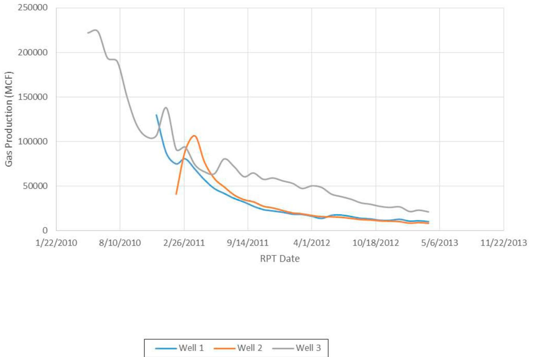
Figure 9. Production data for three deviated wells. Well 2 has an average monthly production of 30.9 MMCF/month while Well 3 has an average monthly production of 80.2 MMCF/month
