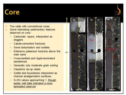
Presenter's notes: This image shows BA-05 core under white light and CT scan. It is a very homogenous rock – sedimentary structures are very well preserved. In BA-05 RCA analysis showed up to 6D of kh. Previous exploration wells had poor log quality and very poor hole conditions (to support Kv/Kh=1).
