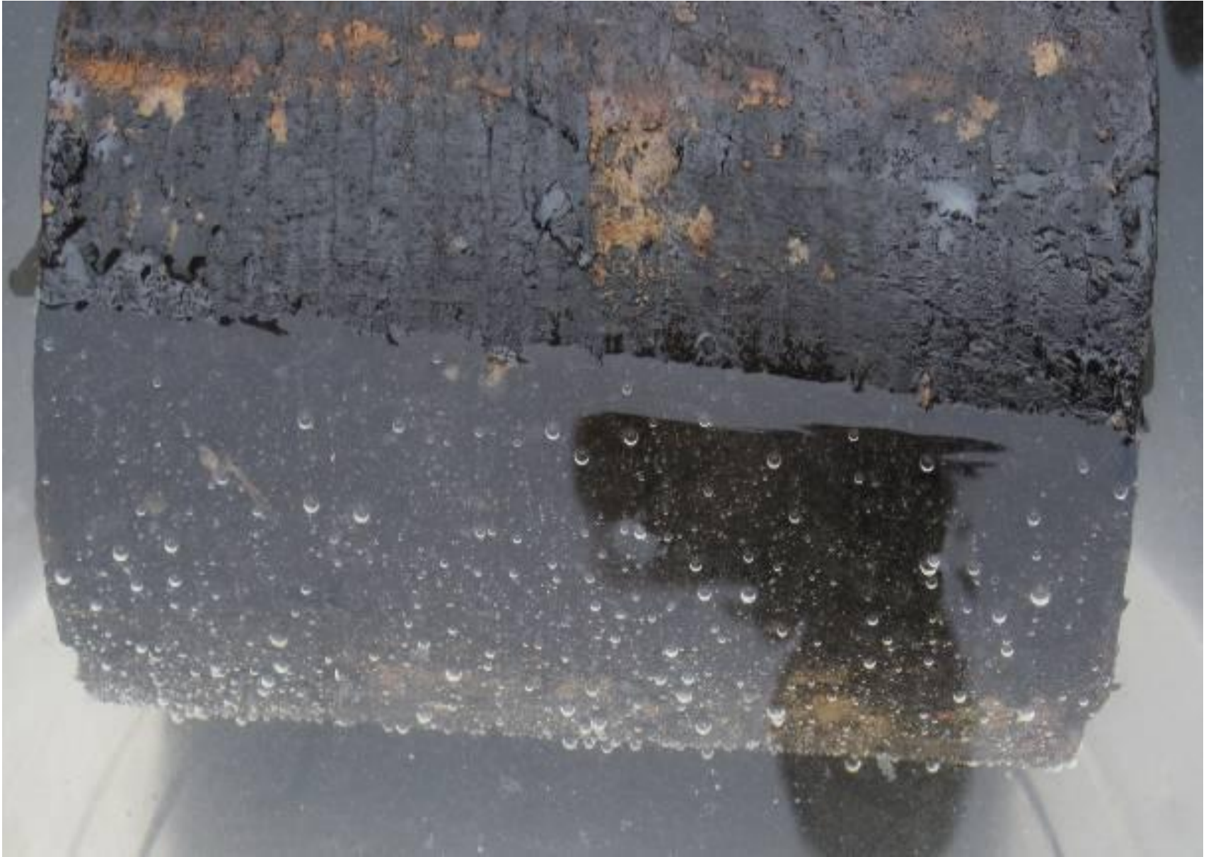
Figure 6. Desorption experiment of Chang-7 Member Shale from Yanye 4 well (1612.3 m).
