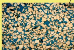
The Cocoa Sand Member is a subangular to subrounded, poor to moderately sorted quartz-rich sandstone with the cleanest sand and most coarse grainsize found at the top of the Member. Yellow bar scale is 250 µm.
