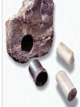
The RSC tool can be used to provide physical samples of the thinly bedded reservoir by acquiring cores perpendicula to the borehole wall. The core is recovered as a cylindrical shaped plug of the formation The core samples will allow important lithological calibration of the NMR and image log data and will provide accurate readings of porosity and permeability. These data will reduce reservoir analysis uncertainty in thinly bedded formations.
