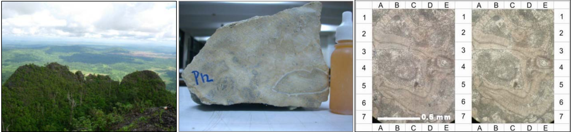
Figure 5. Gentle morphology of carbonate build up facies (left), consist of boundstone; abundant of coral reef fossil which can be seen from slab analysis (middle), thin section photographs shows ornament of coral body (right).
