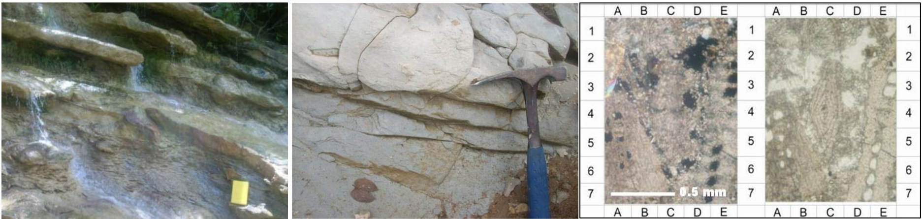
Figure 6. Intercalation bioclastic limestone which consists of mudstone and wacke-packstone (left), mudstone facies which is characterized by very fine grained carbonate sediment (middle), thin section photograph of packstone facies which has abundant foraminifera and other fossils (left).
