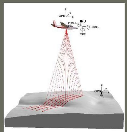
LiDAR means light detection and ranging
