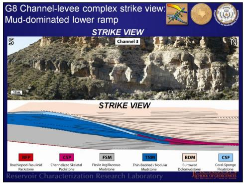
Presenter's notes: This view is up depositional dip through the channel-levee complex present in Last Chance Canyon. The channel system is characterized by mixed erosional and depositional phases with aggradational levees and erosive channels that exhibit minor deposition of packstones in the channel axis.
