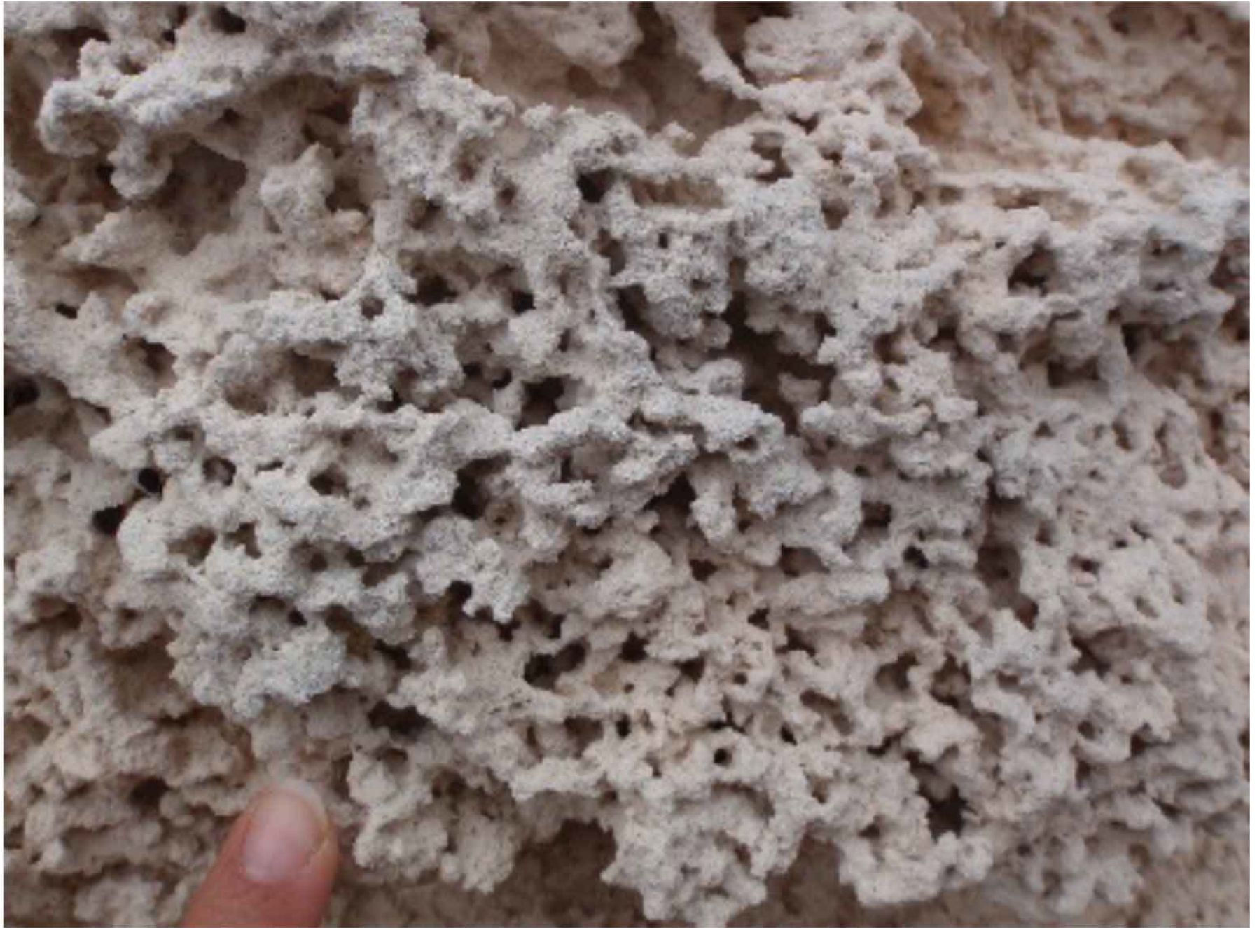
Figure 2. Close up view of the spongiform texture characterized by an intricate network of openings of variable size and morphology.
