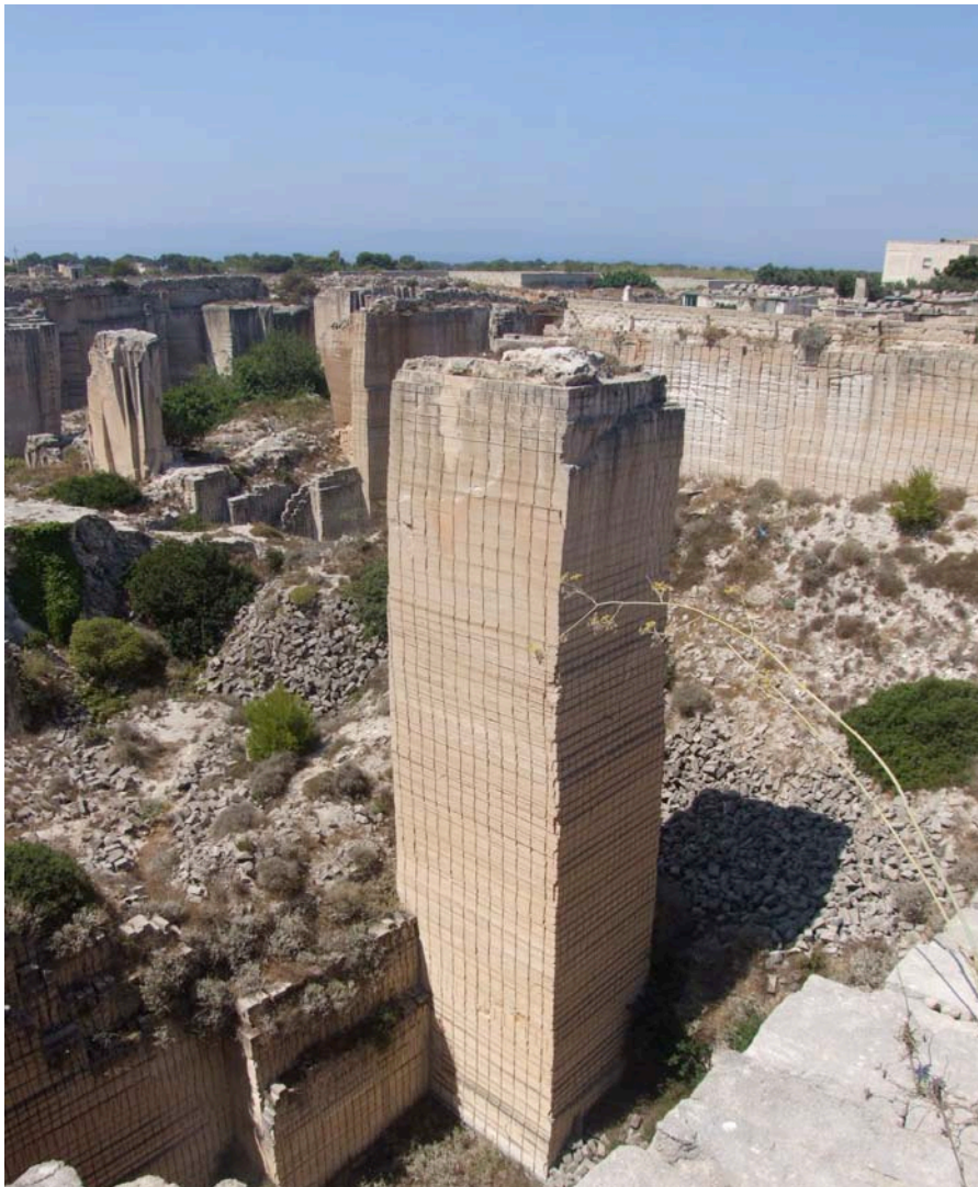
The 'skyscraper': an isolated 4x4x30 m high rocks, spared from quarry exploitation. Just one grid block ?
