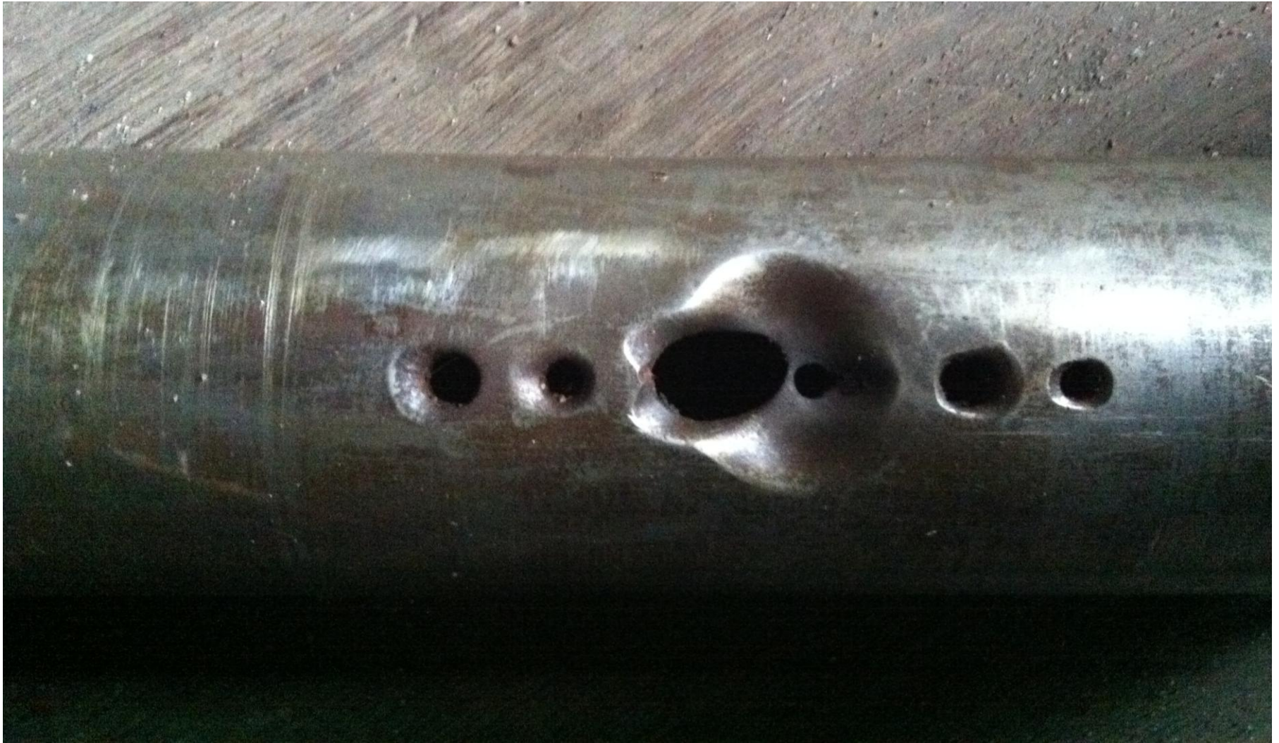
Figure 7. Jet body erosion after 62 perforations performed with 3.06-in. OD (only the enlarged hole is a nozzle).
