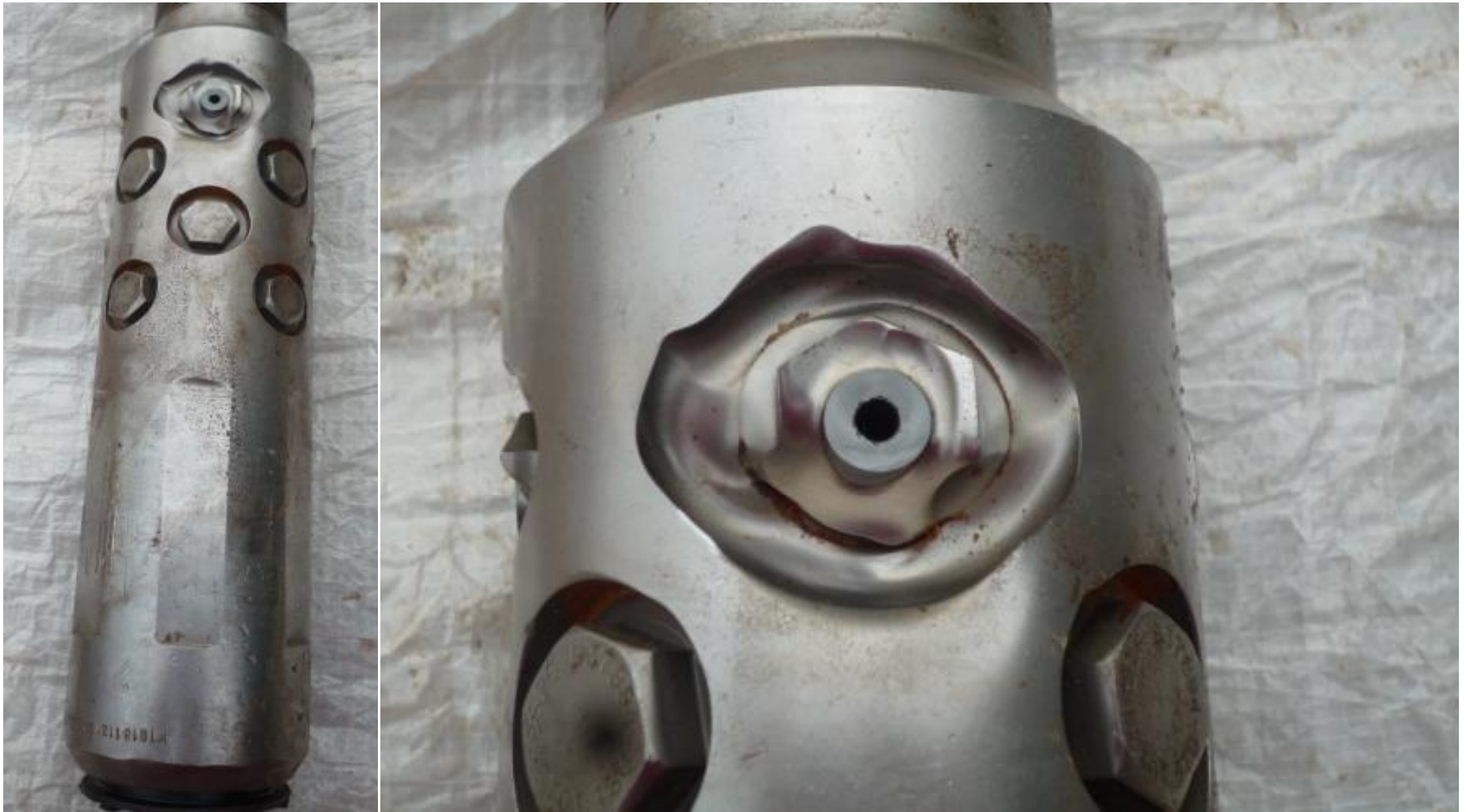
Figure 6. Jet body erosion after 22 perforations performed with 3.66-in. OD.
