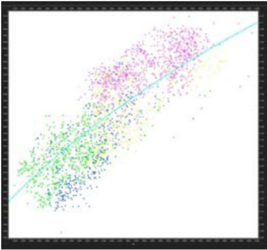
Figure 7. Cross Plot Vp vs Density colored with well Gardner Law: hob=0.31 * Vp^{0.253}
