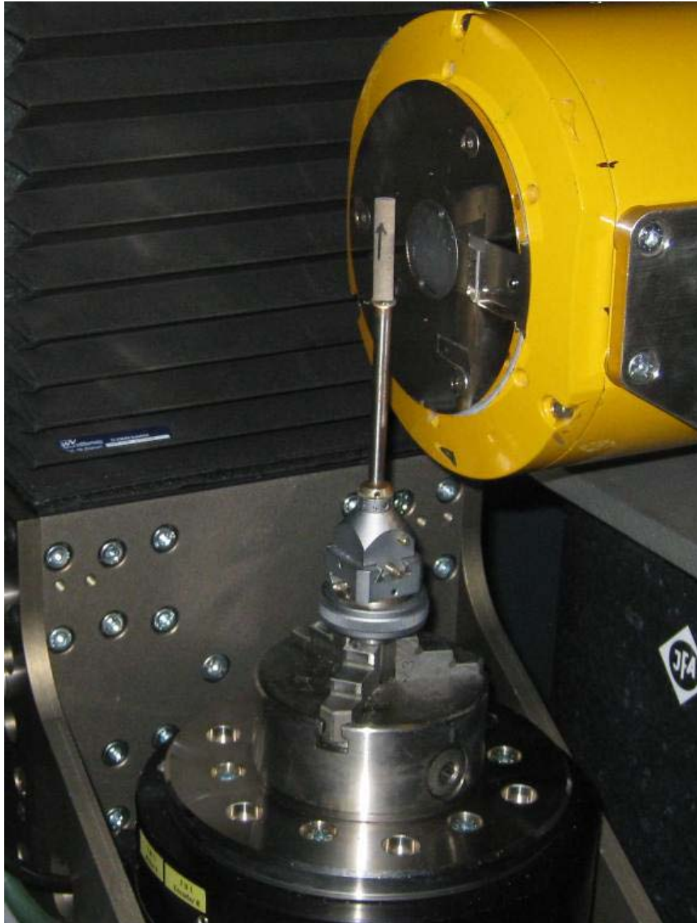
Figure 2: Observation of a carbonate sample in IFP Energies nouvelles microscanner.
