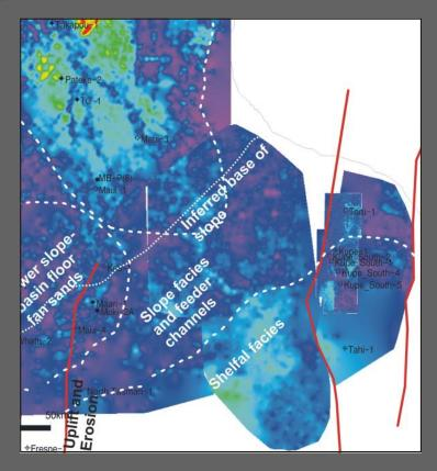
Seismic stratigraphic and attribute mapping (Jan Baur Ph.D.) has been used to constrain paleofacies interpretations.
