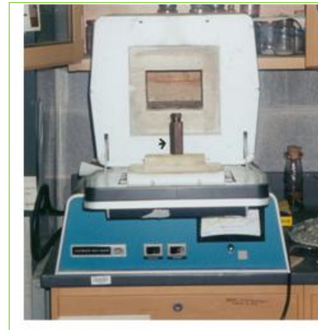
Furnace and sample holder (arrow) used in hydrous pyrolysis experiments
