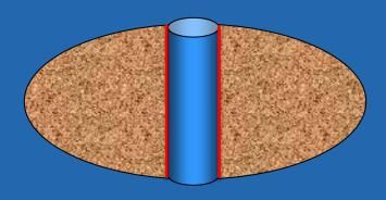
One vertical fracture (100 ft x 150 ft x 1/8 in.) 23,562 ft<sup>2</sup>
