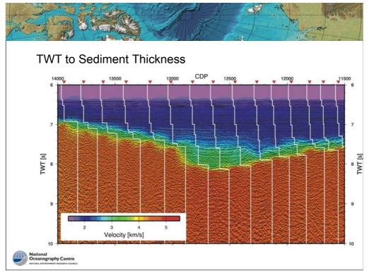
Presenter's Notes: In this slide we show how we measure the thickness of sediment by transferring information of TWT into distance (or thickness).
