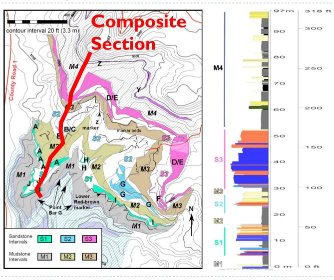
3 Sandstone-rich Intervals containing major sandbodies. Separated BY: 4 Mudstone-rich Intervals: Lower 3 lack Coal, Upper (M4) is coal-rich Capped at top by "coal marker sandstones" correlated to base of Williams Fork by Brownfield et al.. 2000
