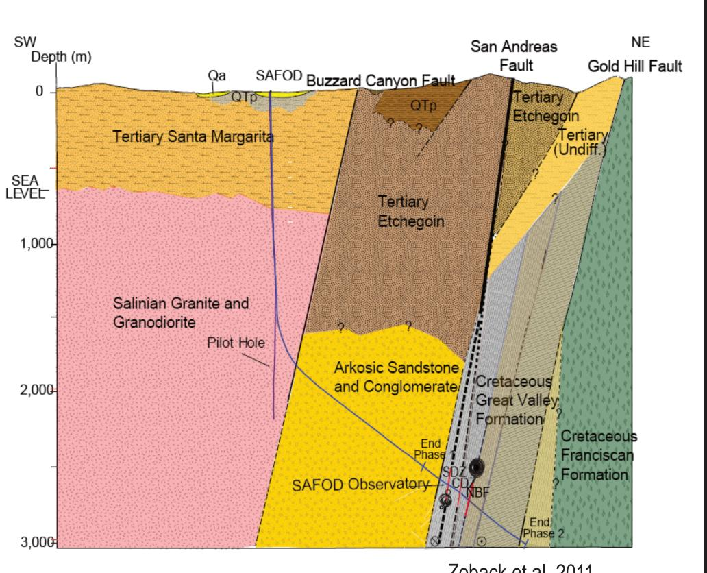
Third-order faults: Fractures and smaller faults identified in the
