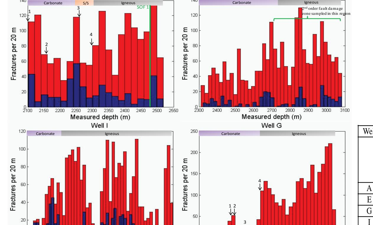
The number of steeply dipping fractures increases very significantly after correction is applied. Well A being a vertical well fails to sample steeply dipping fractures adequately
