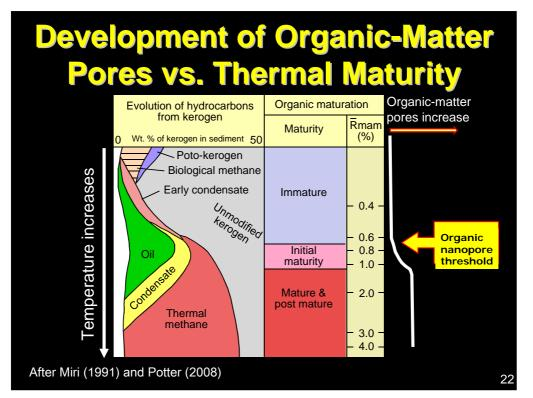
Presenter's notes: Suggests that it may be thermal methane that drives the formation of nanopores, not just any hydrocarbon.
