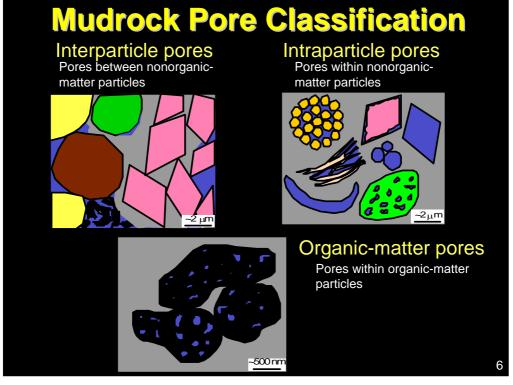
Presenter's notes: We divide mudrock pores into three classes. First we separate pores between pores associated with organic matter and pores not associated with organic matter.
