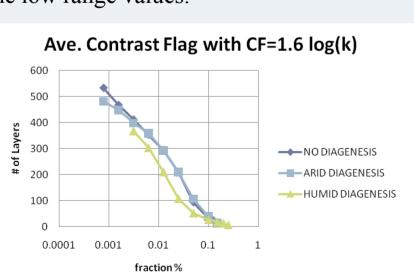
For three of the above contrast methods, amalgamation was implemented for upscaling the 3 full-resolution "truth" models, each of which consisted of 1704 layers each. From the three graphs above and left, the no diagenesis and arid diagenesis models are virtually identical. However the humid climate model reduces to fewer layers on average for all three methods, due the methods ability to capture small perm contrasts.
