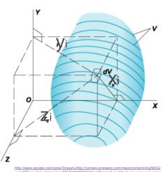
where  $x_i, y_i$  and  $z_i$  are the distances of point i from the coordinate axes. Here the physical meaning of  $I_{xx}$  is the moment of inertia around the x-axis when the objects are rotated around the x-axis and  $I_{xy}$  is the moment of inertia around the y-axis when the objects are rotated around the x-axis.
