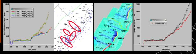
Capturing natural fracture reactivation strongly improved fluid flow modeling
