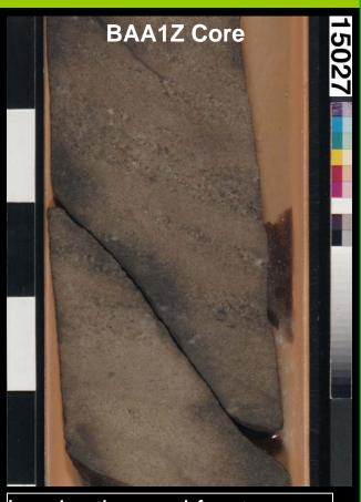
Lamination and fractures create permeability contrast that controls the fluid flow patterns.
