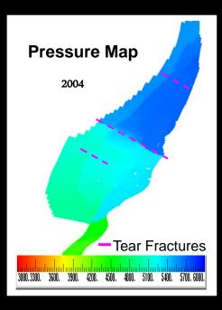
Initially undetected pressure baffles start to become evident and originally sealing faults starts to allow flow across them
