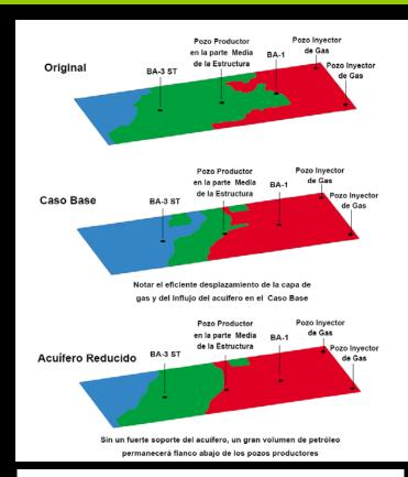
Efficient gas expansion and aquifer support was interpreted
