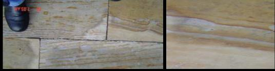
Oxidation shows flow patterns that reflect variations in permeability similar to those observed in cores.
