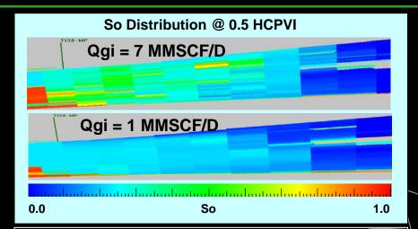
Flow velocity highlights permeability contrasts promoting fingering and reducing the sweep efficiency.
