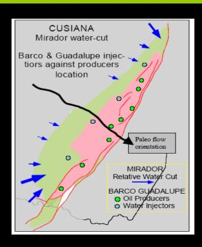
Water breakthrough in all reservoirs does not follow easy to interpret path
