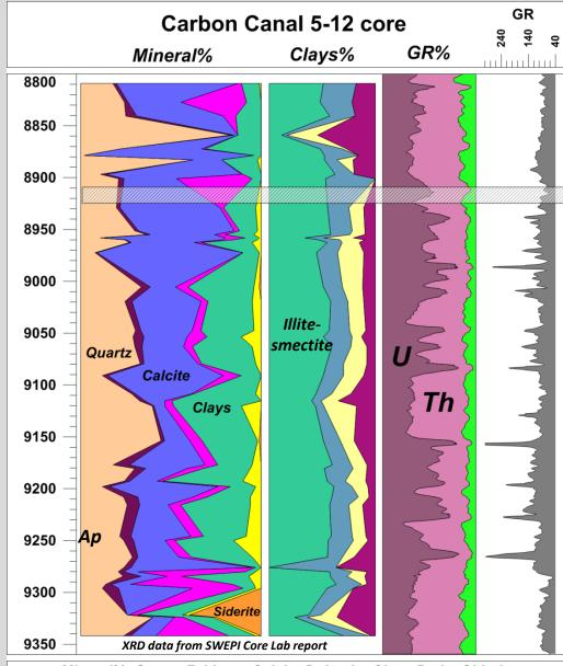
Mineral%: Quartz-Feldspar-Calcite-Dolomite-Clays-Pyrite-Siderite Clay%: Illite-smectite - Illite - Kaolinite - Chlorite GR%: Uranium - Thorium - Potassium
