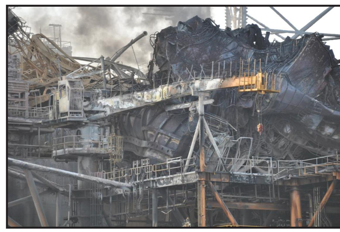
Devastating rig fire due to a blowout believed to result from inaccurate pore pressure prediction.
