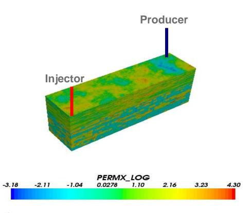
SPE 10 reservoir model, 1,200,000 grid cells (60X220X85), 7.8 Mt CO<sub>2</sub> injected.
