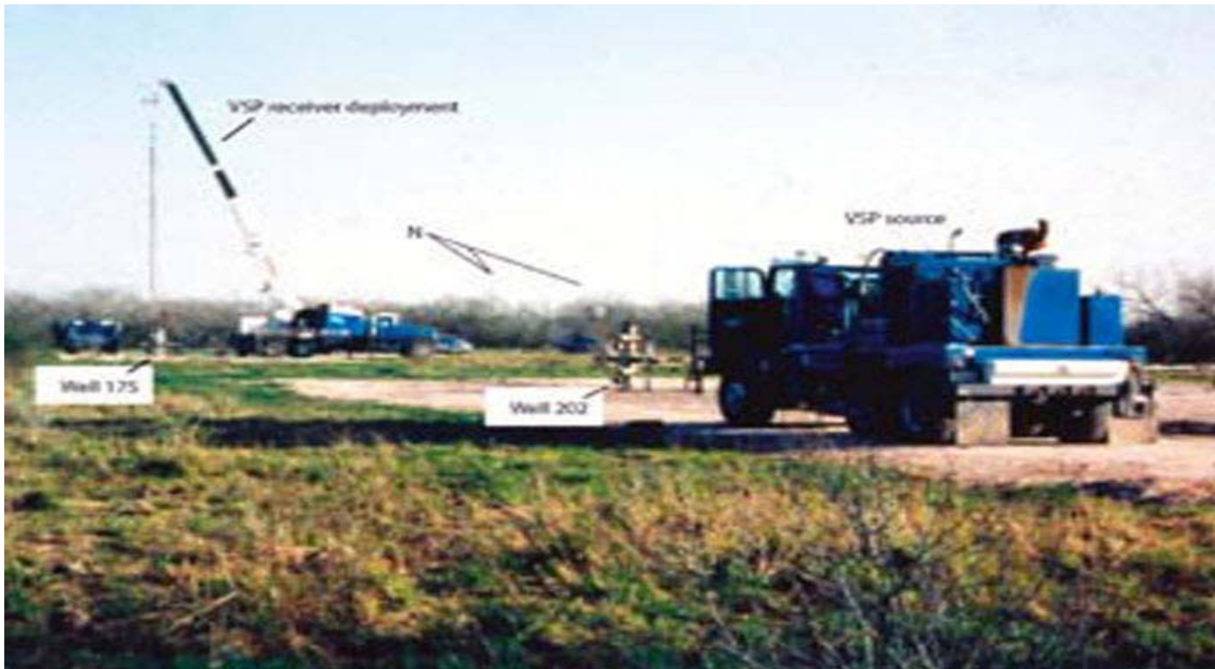
Figure 4. Photo showing the proximity of wells 175 and 202. It is sobering to think a reservoir compartment boundary occurs in the short interwell distance between these two wells. In this photo, a zero-offset VSP is being acquired in well 175. For the data shown on Figure 3 , the receiver system was in well 202 and the vibrator source was far to the north of well 175.
