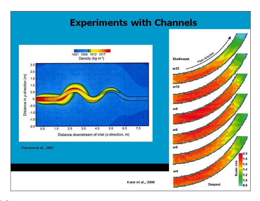
The left image shows early spreading and overbank flow (the densities are shown in a slice just above the channel banks).
