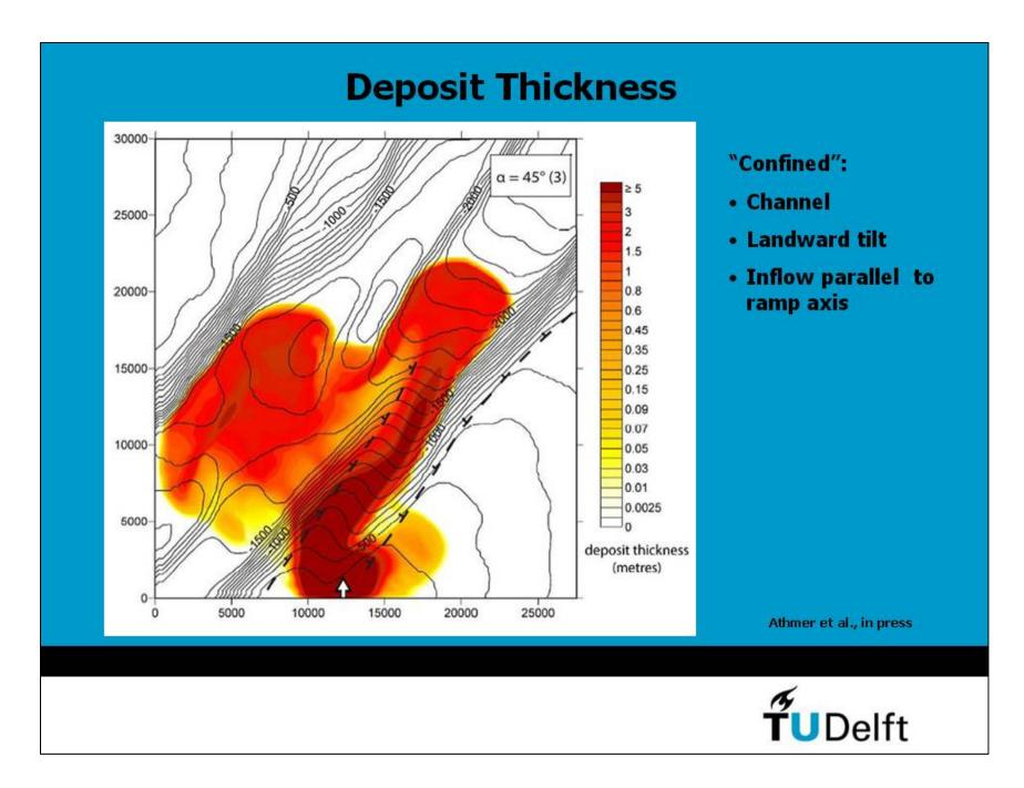
The impression could be that the flow made a U-turn at the base of the ramp. But the flow vectors show otherwise.
