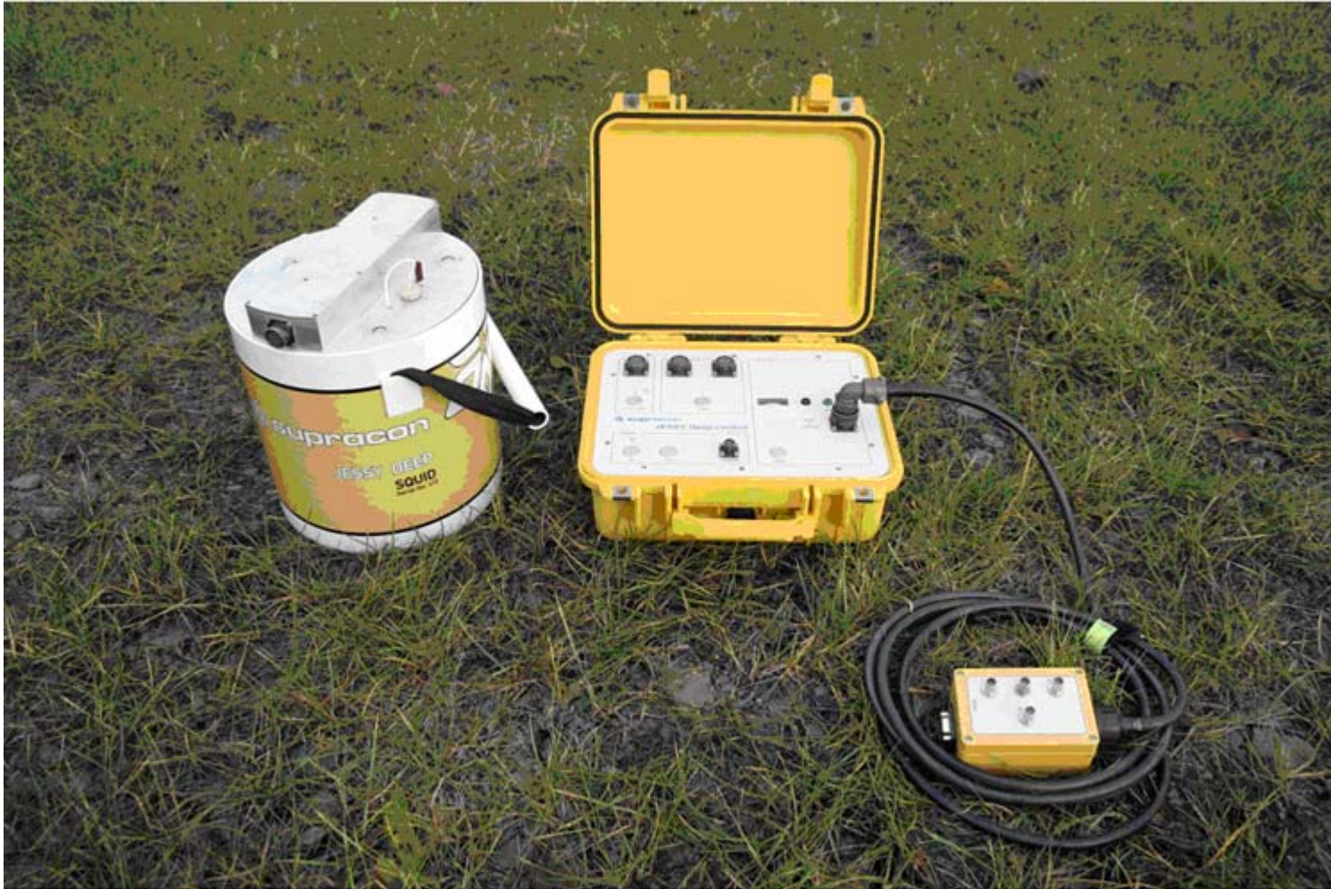
Figure 4. IPHT HTS TEM SQUID system. Left: Cryostat and electronics on top. Centre: Power supply and control unit. Right: BNC adaptor box for laboratory work.
