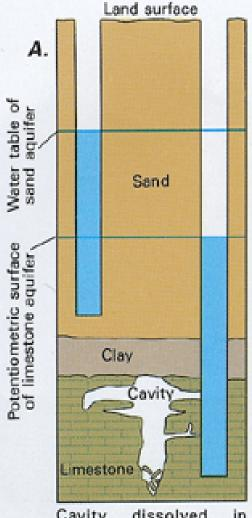
Cavity dissolved in limestone by percolating ground water. Time: Centuries.
