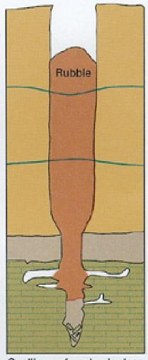
Spalling of cohesionless sand into cavity. Time: Hours to days.
