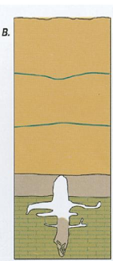
Collapse of overlying clay into cavity by spalling. Time: Months to years.
