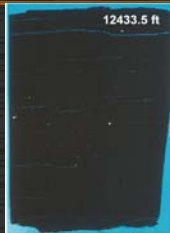
Very thick thin section of compacted laminated mudrock.
