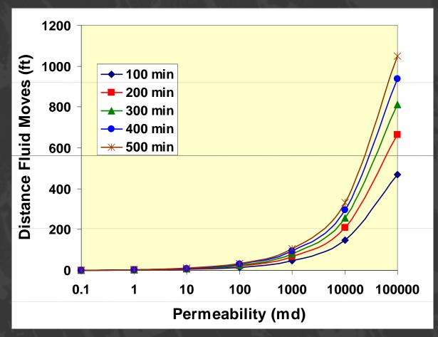
Result: Must Have Hydraulic Fractures In Order To Kill Offset Wells
