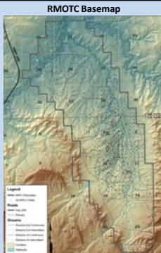
Basemap of NPR-3 using ArcGIS software after GIS Technology implementation at RMOTC. The features here are all tied to the NAD 1983 Wyoming State Plane East Central Zone reference system.
