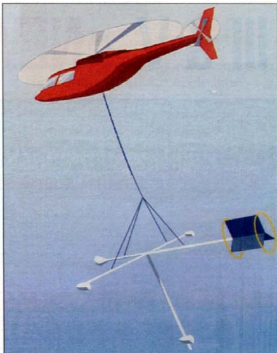
Figure 5. Helicopter-mounted HRAM system. The magnetic platform is suspended at an altitude of 30 meters, enabling the sensor to drape topography in rugged terrain and thus minimize the effect of topographic relief in the magnetic data.
