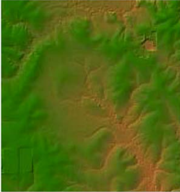
Figure 2. A digital elevation model of LIDAR (Light Detection and Ranging) data from the southwest quarter of the Greensburg 7.5-minute quadrangle; downloaded from the Atlas: The Louisiana Statewide GIS website ( http://atlas.lsu.edu ) and viewed with MacDEM Viewer.
