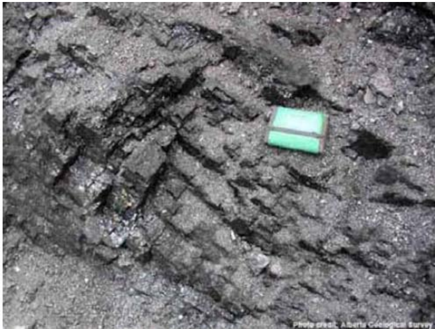
Figure 2. Outcrop showing cleats observed in coal (Alberta Geological Survey). The dominant cleat is oriented from bottom right to upper left and the secondary cleat is perpendicular to it and can be seen to truncate against it.
