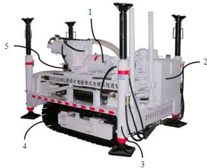
1. Mainframe 2. Power stations 3. Support device 4. Crawler bodywork 5. Control panel
