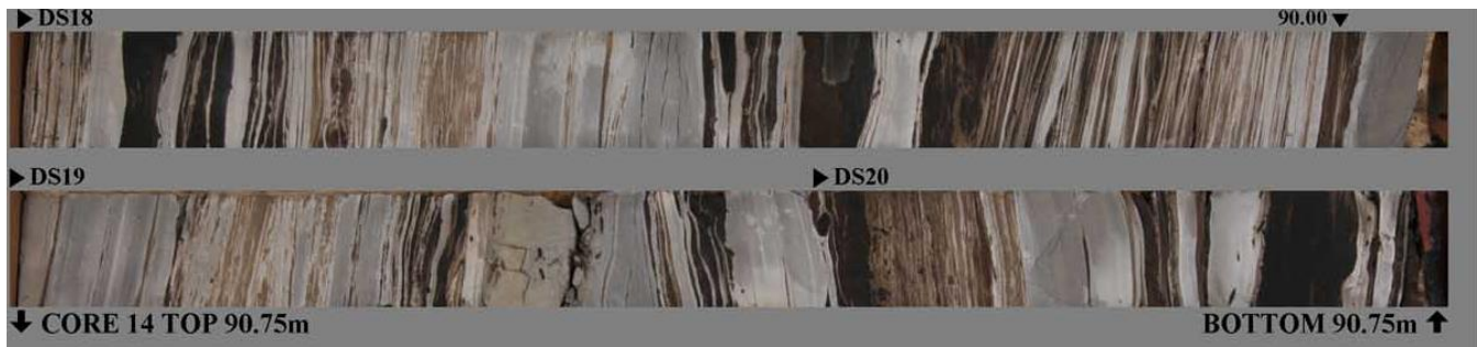
Figure 3- Core logged as SW=1
