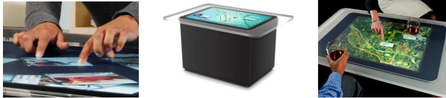
Figure 1: The Microsoft® Surface® 1.0, with support for multitouch interaction, tangible objects on its surface, and multiple simultaneous users.
