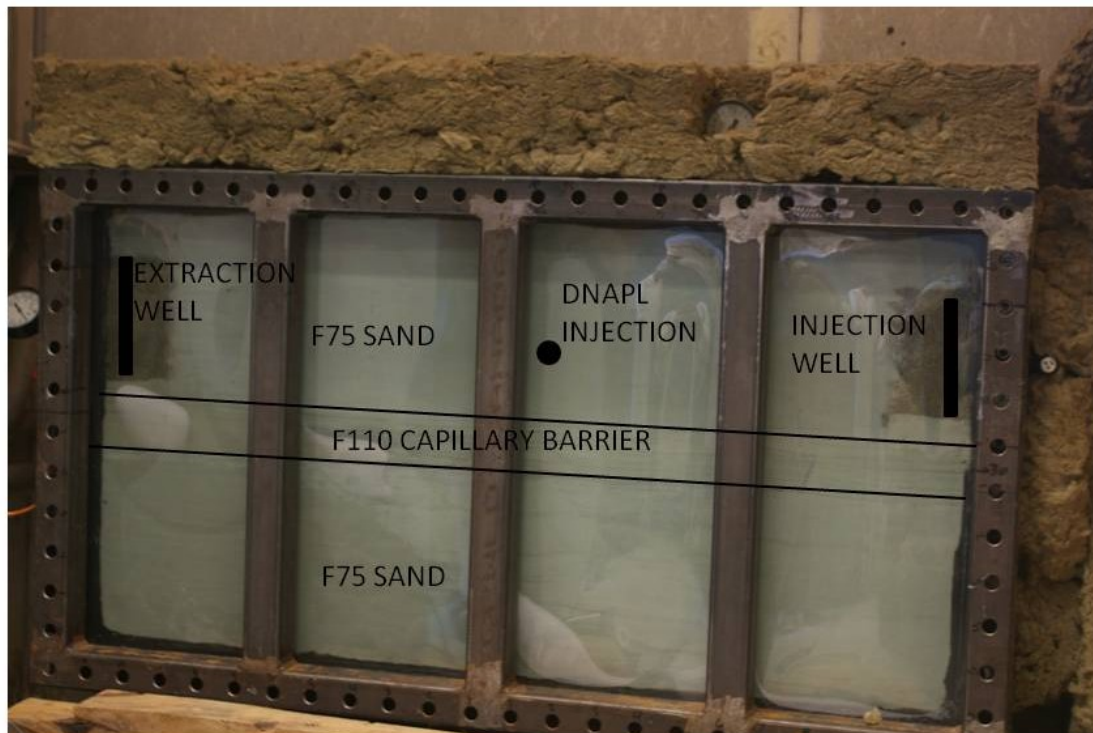
Figure 1: Laboratory cell used for steam flushing experiments
