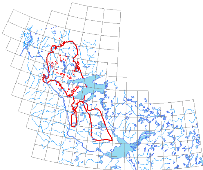
Figure 1: Play map of Cambrian clastic gas play, Interior Platform, Northwest Territories. Closures derived from seismic time-structure maps available in National Energy Board files (Lemieux et al., 2008).
