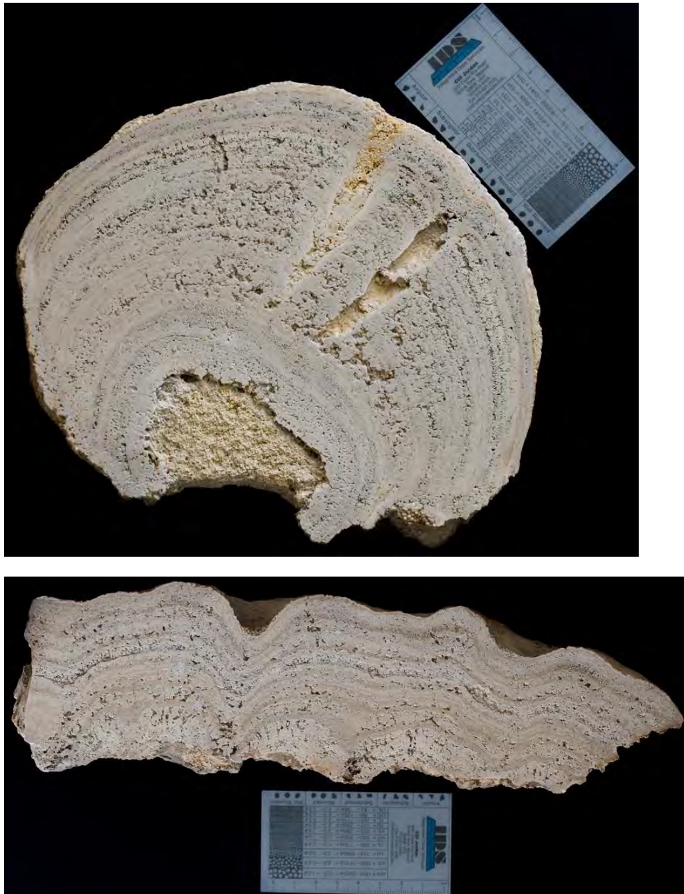
Figure 2. Microbialite mound and polished slabs showing shrub-like thrombolitic and laminar stromatolitic structures. Porosity types include vuggy, inter-shrub, and fenestral. Large tubular vugs are embedment structures.
