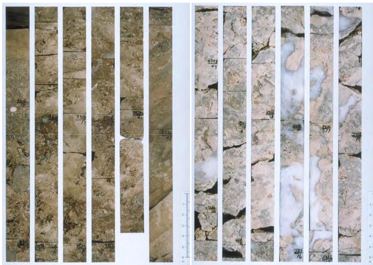
Figure 2. Core photographs of the slope (left) and reef (right) facies from Garber et al. , 1989. The slope from 3512.3 to 3524 ft (1070.5 to 1074 m) contains mostly a possible large talus block from 3513.2 to 3522.2 ft (1070.8 to 1073.6 m) of brown doloboundstone with numerous sediment- and evaporite-filled cavities. Wackestone/packstone beds above and below show inclined bedding. The reef facies from 2308.6 to 2320 ft (703.7 to 707.2 m) is tan to mottled tan-gray doloboundstone with layers of skeletal dolowackestone/packstone and dolograins. Sponges, bryozoans, and microbial forms ( Archaeolithoporella , encrustations, and rare stromatolitic forms) are the principal constituents forming the boundstone texture. Dissolution and precipitation of medium to coarsely crystalline dolomite have obscured, and locally destroyed, primary textures. Early-phase cements, having fibrous, bladed, and botryoidal textures, are present in some cavities (at 2312.7 ft (704.9 m), for example). Note the spectacular cavity-filling gypsum and anhydrite cements.
