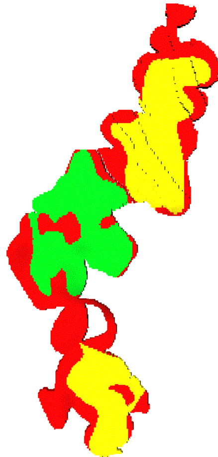
Figure 4: Polygons based on AVO response, indicating reservoir quality in terms of porosity and NTG. green=high, yellow=medium, red=lowest quality.
