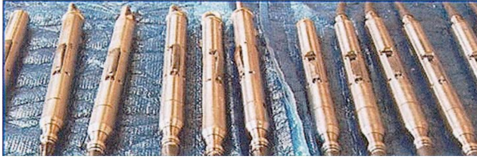
Figure 1. The VSP tool shown above consists of 12 individual sondes linked by an electronic cable and terminated with a logging cable head. The distance between each sonde can be 10, 15 or 20 m. Each sonde contains three orthogonal geophones (two horizontal and one vertical) and a single hydrophone. A hydraulically powered locking arm (shown retracted) ensures that the geophone package is secured against the borehole wall. (Photograph furnished by CGG.)
