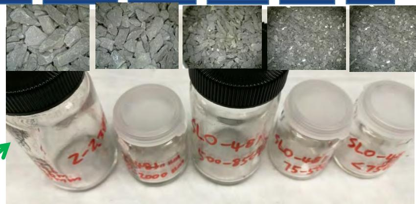
(2) 3 pieces @2-3 cm for thin section, SANS / SAXS wafer, and backup; 5 mm cubes; 4 mm dia. cylinders
