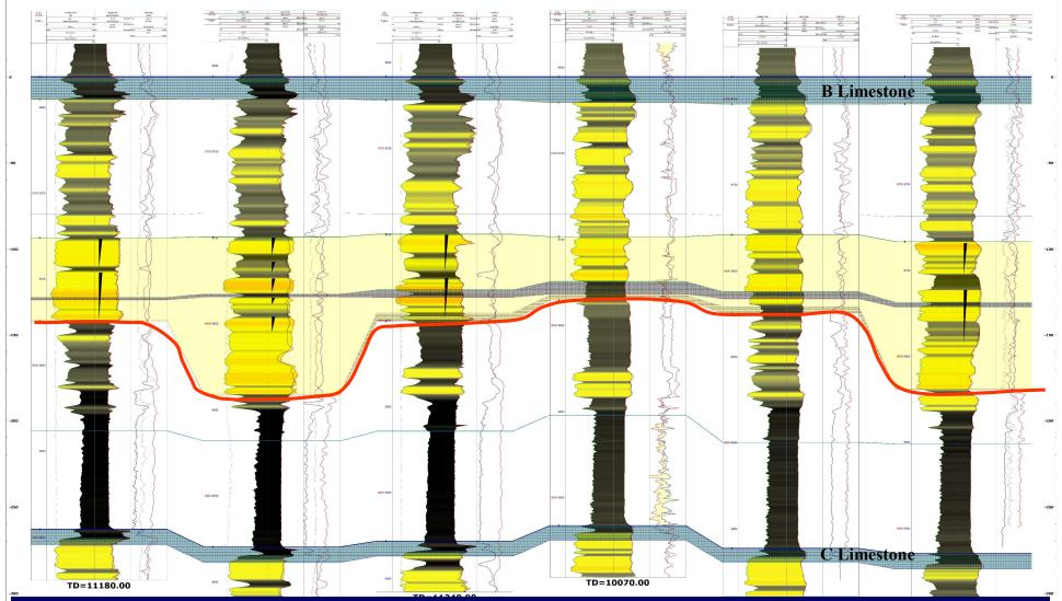
In the Central Oriente Basin, a North-South Napo T Sandstone stratigraphic well log correlation shows that channel development was created by erosion and partial subsidence. Upper T Sandstone shows quartz-glauconitic bars.
