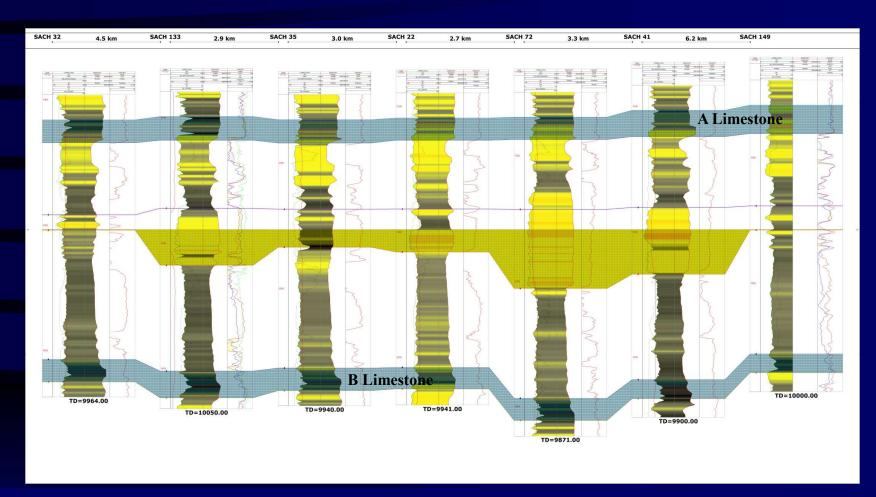
Another example is presented in a North – South stratigraphic well log correlation along Sacha Field, which shows that channel development was created by a combination of tectonic subsidence and partial erosion. A NW-SE fault system generated the accommodation space which preserved sandy facies of Napo U channels.
