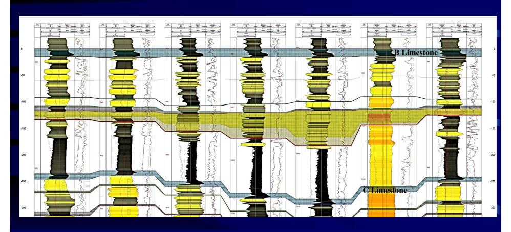
A regional West-East Napo T Sandstone stratigraphic well log correlation running west to east across Paraiso, Inchi and Sacha Fields clearly shows the lateral thickness variation. The A to B Limestones thickness increases related to the Main T Sand channel development, indicating that tectonic subsidence was the main mechanism to create the accommodation space to preserve sand channels.
