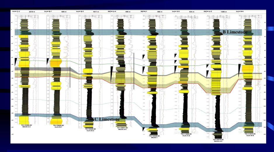
Inchi Field, a stratigraphic play, since no structural closure can be identified (structural nose) shows that the sand channel development is related to mainly tectonic subsidence.
