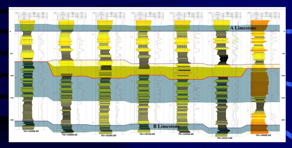
Southwards from present day Napo River, a North – South stratigraphic well log correlation along Auca Field shows that channel development was created by erosion and minor subsidence. A NW-SE fault system generated the accommodation space which preserved sandy facies of Napo U channels. Upper U Sandstone shows quartz-glauconitic shoals.
