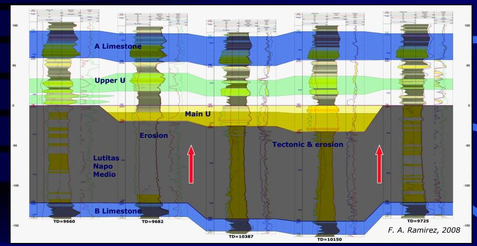
Similar models were later generated for other fields like Huachito, where erosion was combined with tectonic subsidence to generate the space to accommodate the sand channels. The stratigraphic well log correlation shows that sand channel development is related to thickness incremental between the two flooding markers, A and B Limestone.
