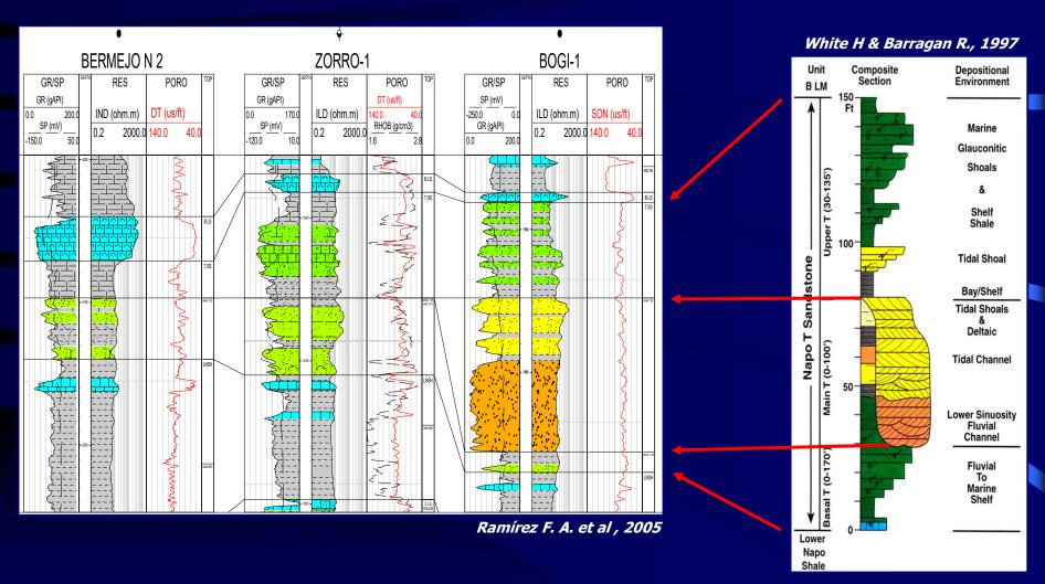
Regional well log correlations, core descriptions and field geology, has allowed to identify three units in the T Sandstone Unit: Basal T, Main or Lower T and Upper T. Each unit show specific facies and lithologies that can be recognized across the Oriente Basin.
