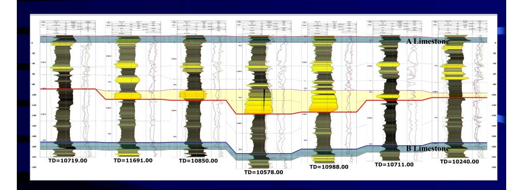
Further to the east, a regional West – East stratigraphic well log correlation across Sacha-MDC-Paka Norte Fields shows that channel development was created by a combination of tectonic subsidence and partial erosion. A NW-SE fault system generated the accommodation space which preserved sandy facies of Napo U channels. Upper U Sandstone shows quartz-glauconitic bars.
